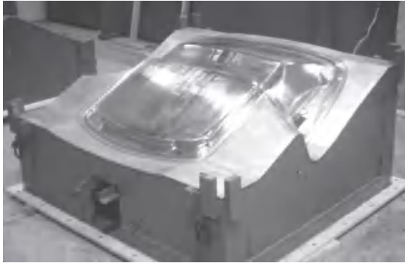
Figure 12 Electroformed nickel mould for reinforced plastic automotive body component
