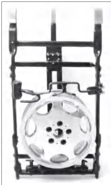
Figure 18 Plating rack specifically designed for automotive wheels
