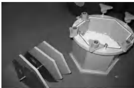
Figure 21 Typical hexagonal tumbling barrel (right) used in the wearing of coated articles suspended between 2 plates of the retaining assembly (left).
