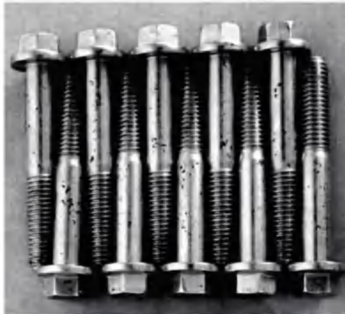
d)Black spots after 240h NSS test of fasteners with iridescent passivated zinc layer
