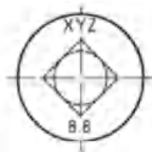
Figure 13—Example of marking cup head square neck bolts
